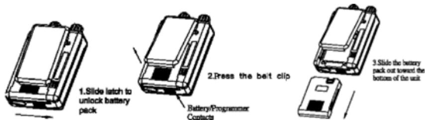
**CAUTION:** If the batteries are improperly installed, the alert monitor will not function and the batteries will not charge.
